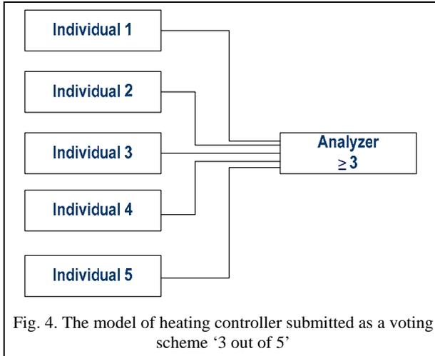
Fig. 4. The model of heating controller submitted as a voting scheme ‘3 out of 5’
