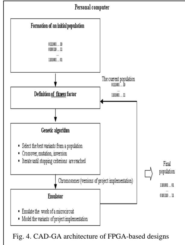
Fig. 4. CAD-GA architecture of FPGA-based designs
