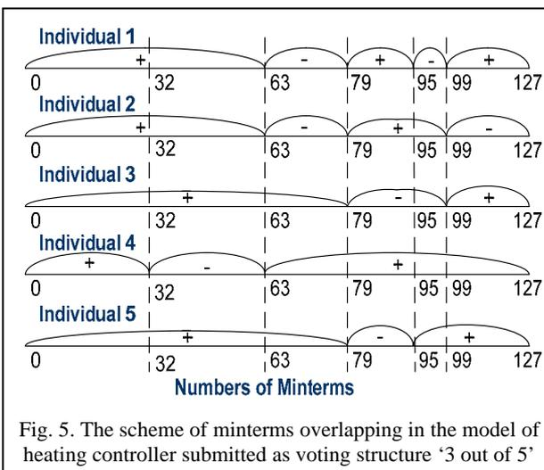
Fig. 5. The scheme of minterms overlapping in the model of heating controller submitted as voting structure ‘3 out of 5’
