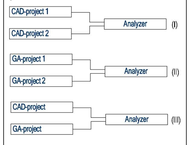
Fig. 2. Internal (I, II) and external (III) FPGA-guided diversification
