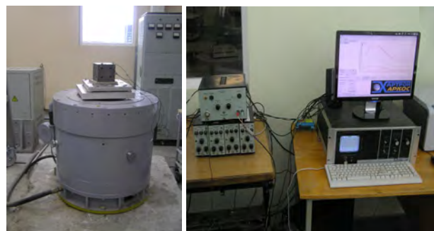
Fig. 1. Equipment of UVE-100/5-3000 for testing on broadband random vibration
