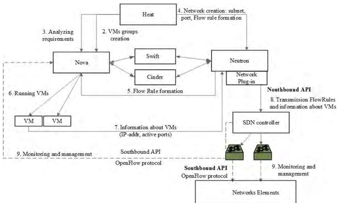
Fig. 1. Interaction process between SDN controller and Neutron
