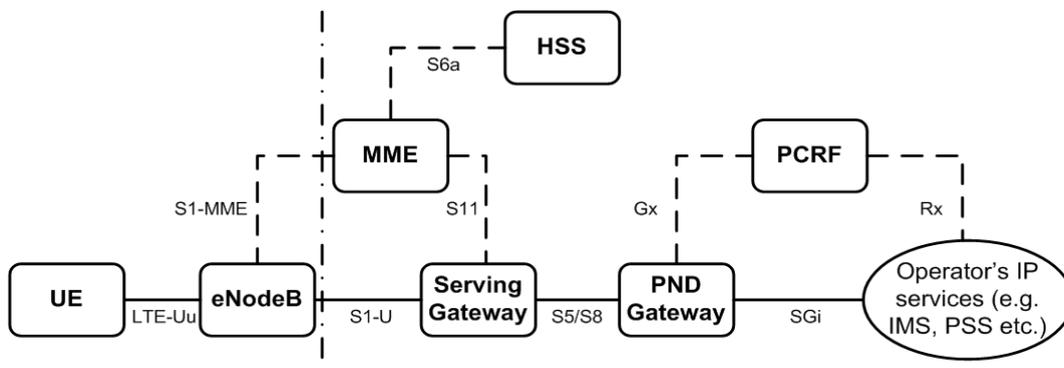
Fig. 1. The EPS network elements
