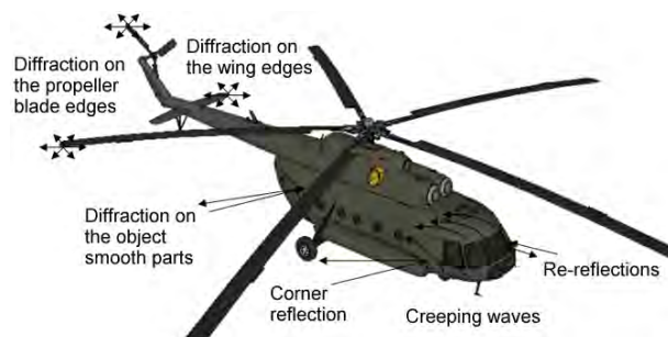
Fig. 1. Most common EMW scattering ways in a helicopter
