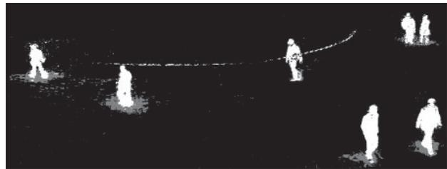
Fig. 2. Foreground mask obtained using MOG2 Background Subtractor
