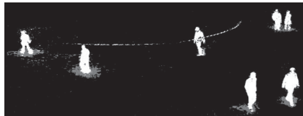
Fig. 2. Foreground mask obtained using MOG2 Background Subtractor
