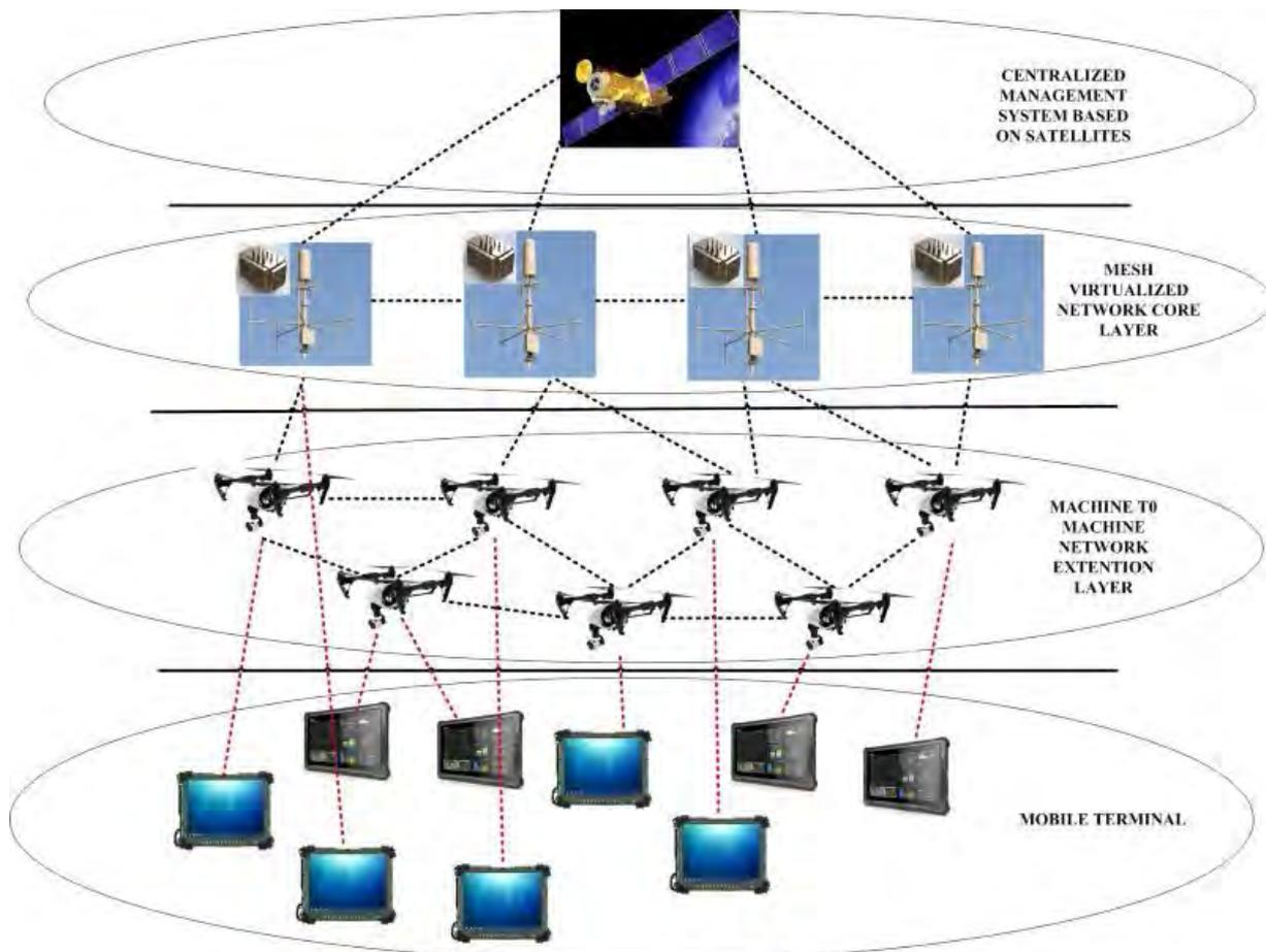
Fig. 1. The concept of military wireless communication system
