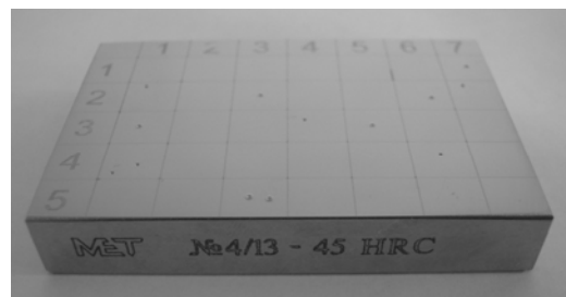
Fig. 2. Layout of the grid on the measurement surface of the hardness reference blocks with the logo
