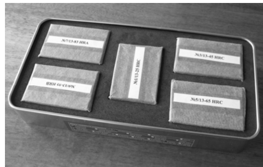
Fig. 1. Rockwell’s set of hardness reference blocks
