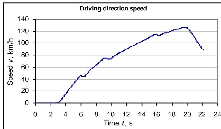
Fig. 4. Calculated car speed with gear changes
