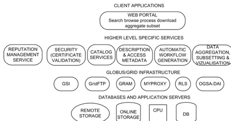
Fig. 3. System architecture
